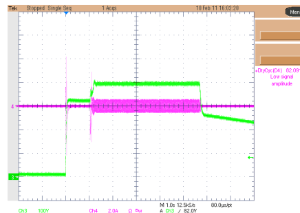
Turn ON delay ~ 1sec @ 230Vac
