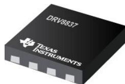
2.0 x 2mm, 8-pin WSON package 2.0 x 2mm, 8管腳 WSON封裝
