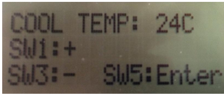
Figure 37: Setting Cooling Setpoint on SampleThermostat
