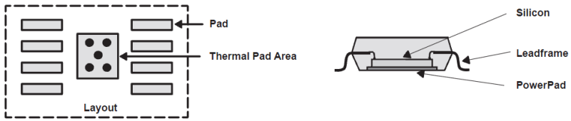
Figure 6. PowerPAD™ Improves Heat Sinking
