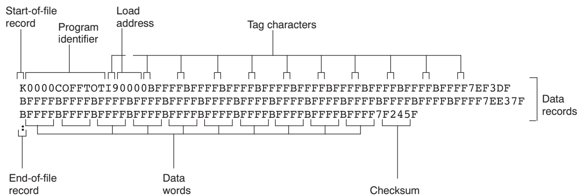
Figure 12-13. TI-Tagged Object Format
